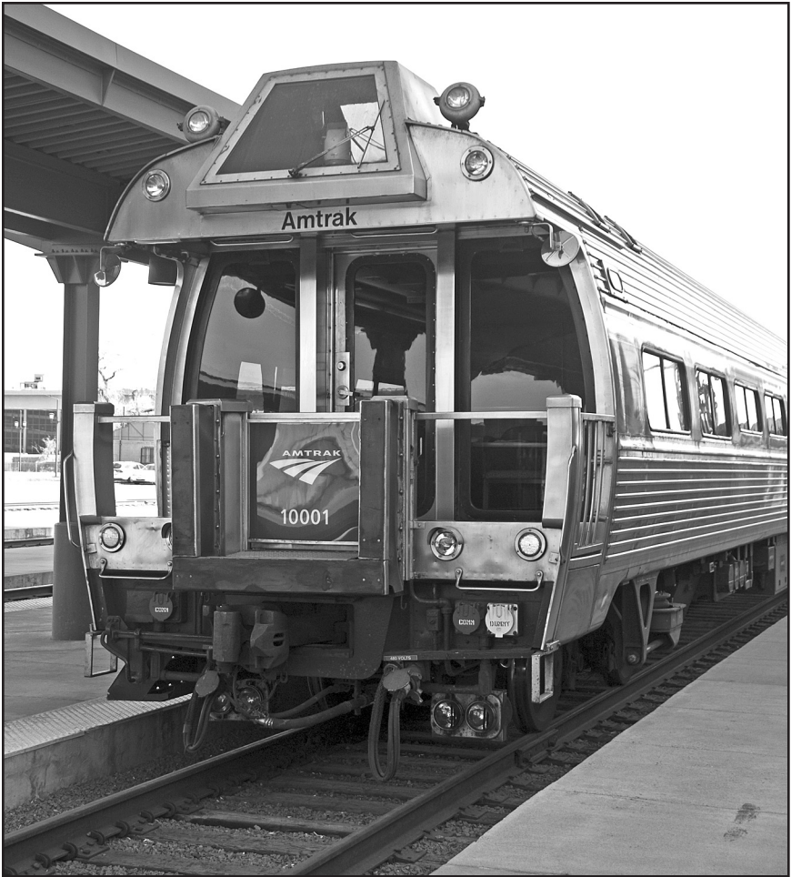
Amtrak business car 10001 - BEECH GROVE - Denver Union Station, 4/16/08. Note camera in enclosure mounted over rear platform. Wind shield wiper helps camera visibility along with all the rear facing lights. – Photo © 2008 by Chip.
